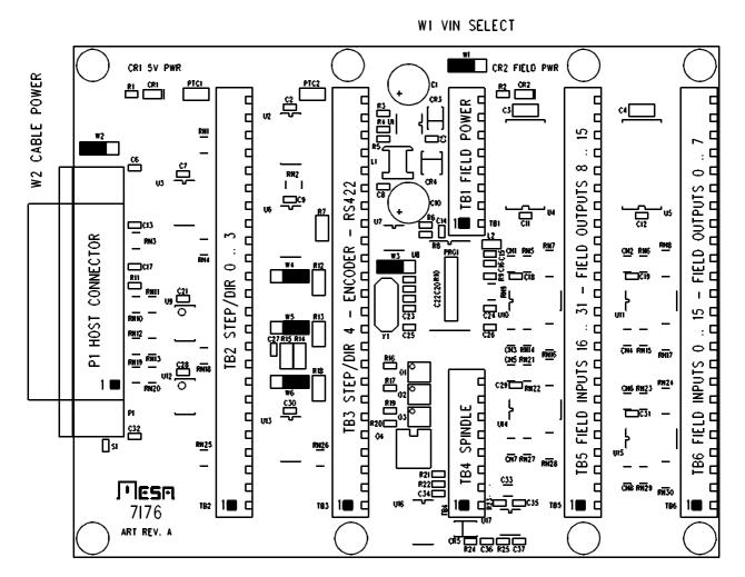
NOTE: TERMINAL BLOCK PIN 1'S ARE MARKED WITH SQUARE PAD
